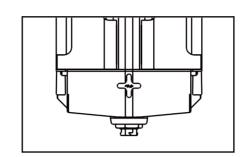
(3) Loop the waterfall mounts on the wire deck or cross bar. Slightly separate the mounting hardware until the hooks slide into the holes on the side of the power supply enclosure.
