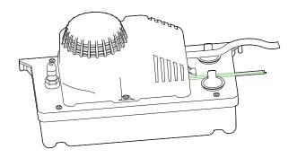
Step 2 Open the cover. You will see the water pump has two switches: the pump switch controls pump automatic start and stop; the safety switch can be connected to the external alarm or to disconnect the power supply of condensing equipment as is necessary.
