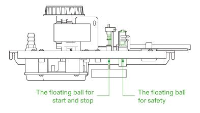
Step 4 There are two methods of wiring the safety switch: the factory default is wired as the electrical parameters of the switch: 5A 250V, the diagram below shows the shape of the alarm switch.
