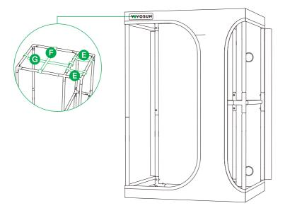
**STEP 11** Pull the zippers to close the walls and door of the tent. Ensure the tent coat fits the frame at the corners.
