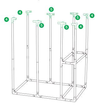
STEP 7 Connect eight (A) Poles to the Corner Supports (4) and Four-way Connectors (5) as shown. Then connect two (D) Poles to the Corner Supports (4) and Four-way Connectors (5) as shown.
