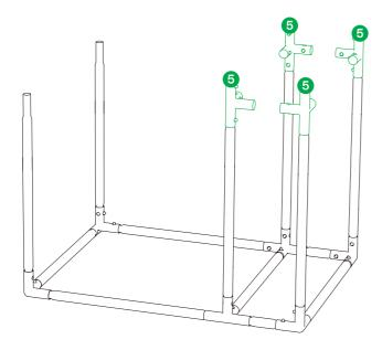
STEP 4 Connect two (A) Poles and two (D) Poles to the Four-way Connectors (5) on the (B) Poles as shown below.
