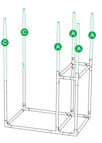
STEP 6 Attach four Corner Supports (4) and two Four-way Connectors (5) to the poles in the correct positions as shown below.
