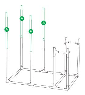
STEP 4 Connect two (A) Poles and two (D) Poles to the Four-way Connectors (5) as shown.
