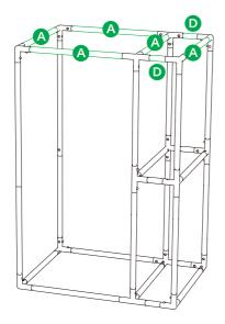
STEP 8 Unzip and unfold the Tent Coat (1). Put the base frame inside it as shown. Ensure the tent coat fit the floor and roof appropriately.
