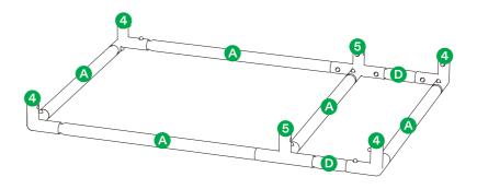
STEP 2 Connect two (A) Poles and four (B) Poles to the Corner Supports (4) and Four-way Connectors (5) in the correct positions as shown below.
