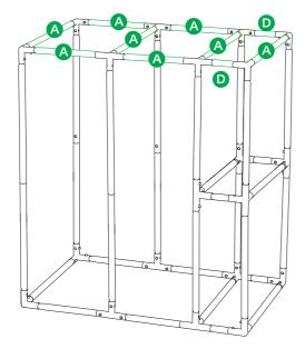
**STEP 8** Unzip and unfold the **Tent Coat (1).** Put the base frame inside it. Ensure the tent coat fit the floor and roof appropriately.
