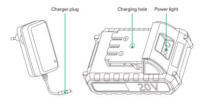
**WARNING:** Fire Hazard. When unplugging the output plug from the charging hole, be sure to unplug the charger from the outlet first and then disconnect the charger output plug from the charging hole.
