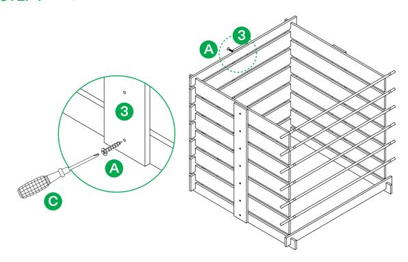
**STEP 8** Prepare 6 x Part 2, then place and assemble them according to the diagram.
