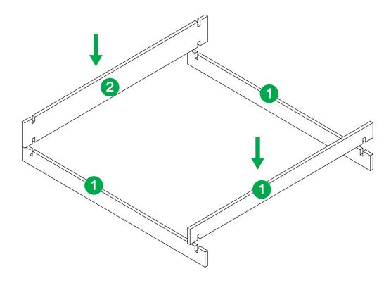
**STEP 2** After completing Step 1 assembly, prepare 2 x Part 3, 2x Part A and 1x Part C, and then assemble them as shown.
