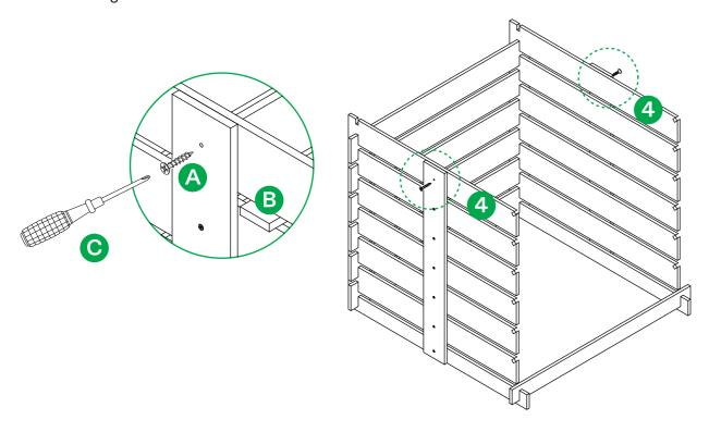
**STEP 6** Prepare 1 x Part 1, and assemble them according to the diagram.
